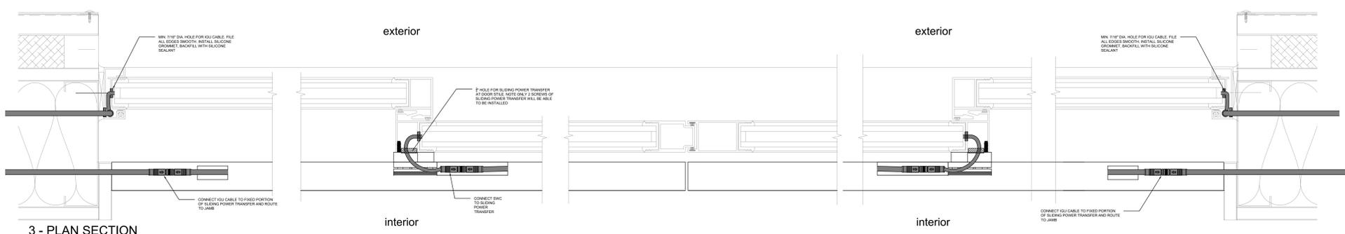
ELEVATIONS AND DETAILS - KAWNEER 1010 SLIDING DOORS WITH SLIDING POWER TRANSFER
